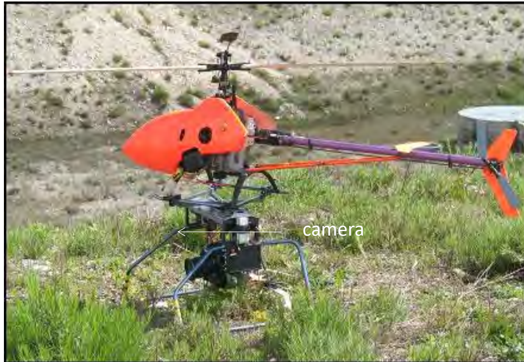
Drone Helicopter-controlled radio (collaboration with MAP-ARIA, EAL)
